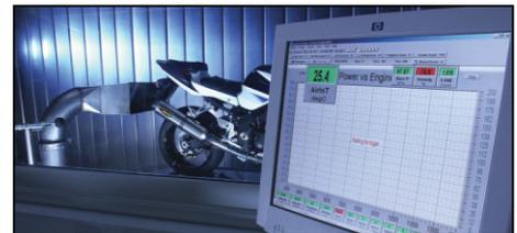
“A new exhaust system is tested up to 200 times before we put it on the road for the first time,” explains Igor. “This test takes place in the dyno benches where we bring the motorcycle up to a speed of 120 km/h to measure the performance as well as the sound. This we do to form the platform for the benchmarking as well as for correlation testing to support the product development team. We have been part of 29 world championships and were awarded best brand of the
